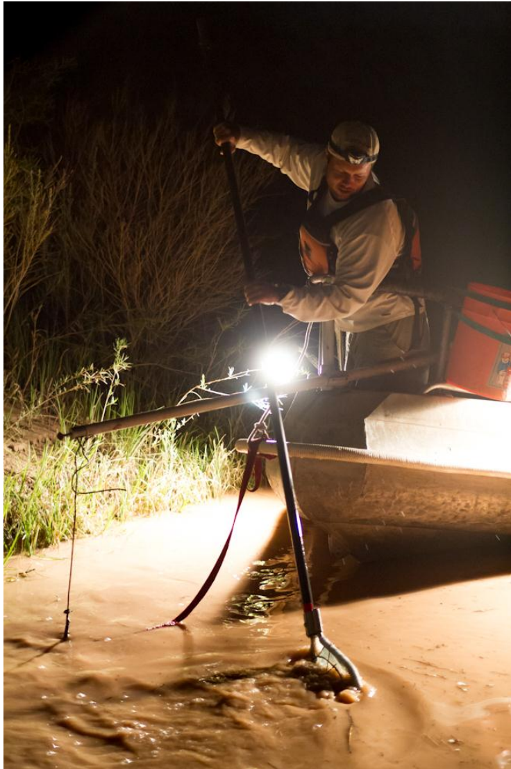
Figure 5. Capturing fish using electrofishing gear, which temporarily stuns fish by passing an electric current through the water. Stunned fish are netted and placed in tanks where they quickly revive.
